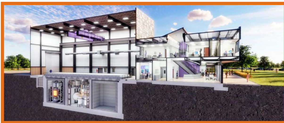
Above: A conceptual rendering showing a section view of the molten salt research reactor along with supporting systems and a simulator room for training students at Abilene Christian University. (Image: ACU)
